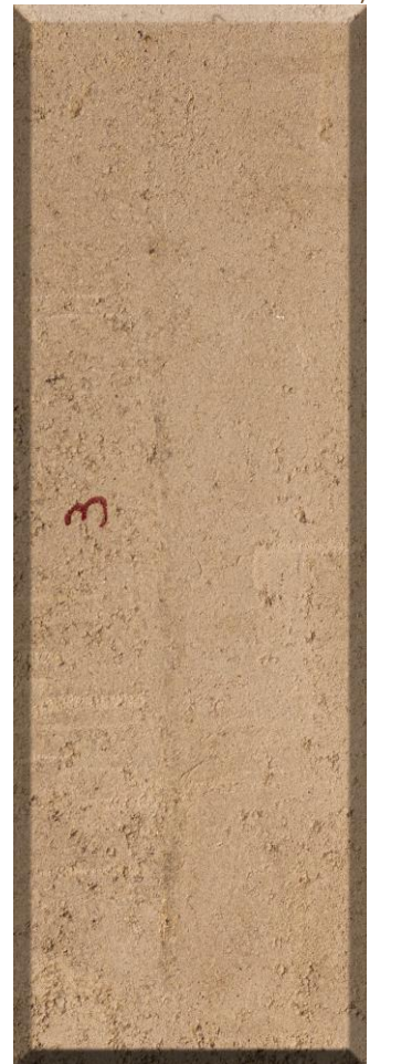
Figura 109 PC_02. Panel 5% de cemento (90x30x6 cm).
