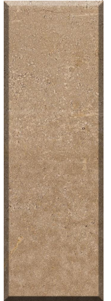
Figura 110 PC_03. Panel 10% de cemento (90x30x6 cm).
