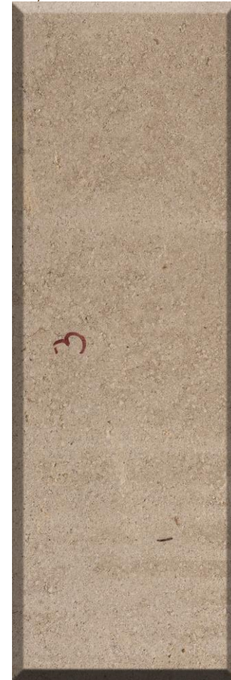
Figura 112 PC_05. Panel 20% de cemento (90x30x6 cm).
