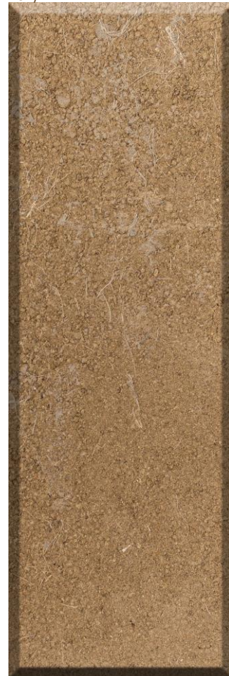
Figura 107 PF_01 - PF_05. Panel 1% de fibras (90x30x6 cm).
