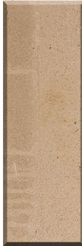
Figura 111 PC_04. Panel 15% de cemento (90x30x6 cm).
