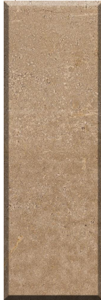
Figura 110 PC_03. Panel 10% de cemento (90x30x6 cm).
