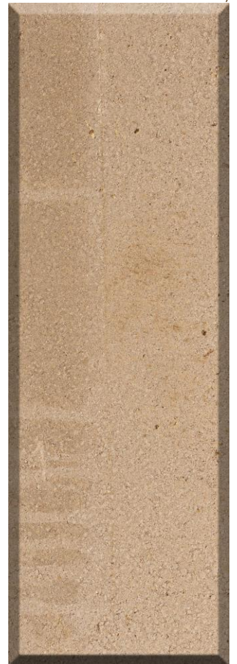
Figura 111 PC_04. Panel 15% de cemento (90x30x6 cm).
