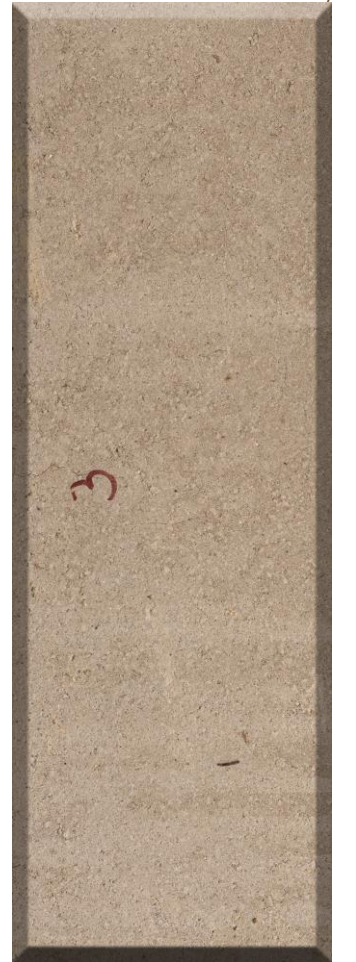
Figura 112 PC_05. Panel 20% de cemento (90x30x6 cm).
