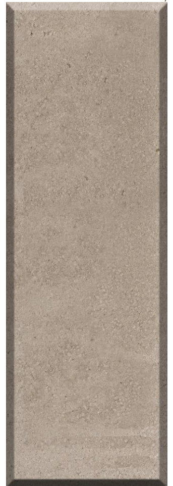
Figura 113 PC_06. Panel 25% de cemento (90x30x6 cm).
