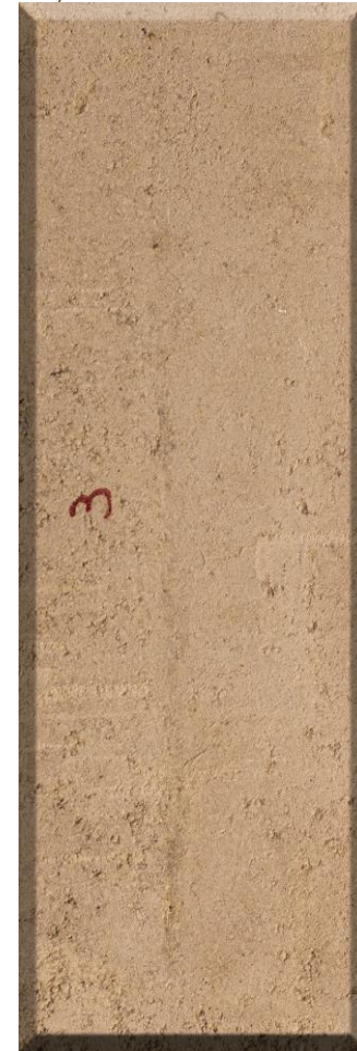
Figura 109 PC_02. Panel 5% de cemento (90x30x6 cm).
