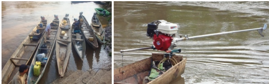
Fig. 7.5 (Left) Traditional canoes, (right) traditional outboard motor “peque-peque”. Source: Ordóñez and Guaman (2014)
